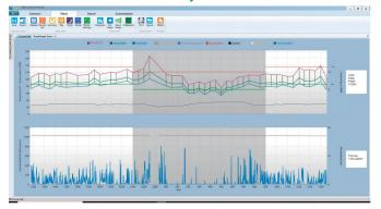
The newly designed software can analyze environmental data collected by the multi-sensor in addition to ABPM measurement data. Temperature, pressure and activity can be graphed alongside blood pressure. TM-2441 only (TM-2440 does not have a multi-sensor)
